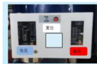
6. If the machine is equipped with a pressure controller, when the compressor does not start, check whether the low pressure value is lower than 0.2MPa, (possible leakage of fluorine), and the filth blockage of the condenser may cause bad heat dissipation in case of higher than 0.2MPa. After the troubleshooting, the red reset button in the ring is pressed
